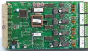
MIRFO Linking interface between a Maylis central and two other Maylis networks through an optic fiber REF 440.3800
